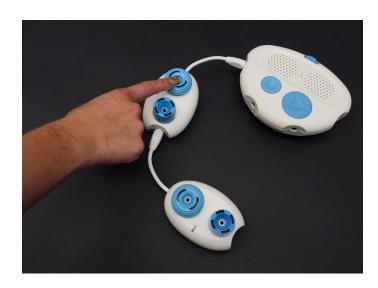
[Figure Caption:] This is a photo of the Code Jumper Hub and two Play pods. One Play pod is connected directly to the Hub at Port 1, and a second is connected to the opposite end of the first Play pod. A child's hand is pointing to the first Play pod, indicating tracing the code.
