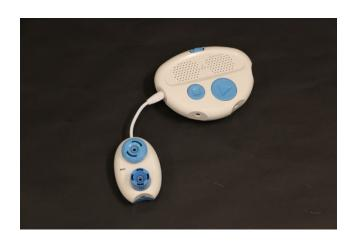
[Figure Caption:] A photo of a Play pod connected to the Code Jumper Hub at Port 1
