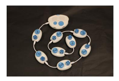
[Figure Caption:] This is a photo of the Code Jumper Hub and eight Play pods. One Play pod is connected directly to the Hub at Port 1, the second Play pod is connected to the opposite end of the first Play pod, the third is connected to the opposite end of the second, and so on.
